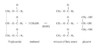
Where  $R_1$ ,  $R_2$  and  $R_3$  are long hydrocarbon chains sometimes called fatty chain.
