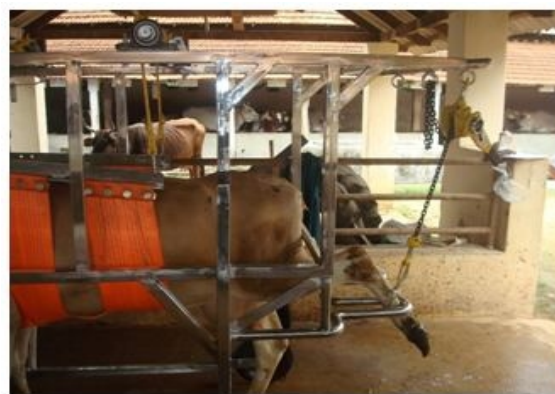
Fig. 2 The animal restrained in the cattle-crush and the entire weight of the animal was supported by the abdominal belt
